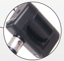
LED and digital camera integrated in wrist
